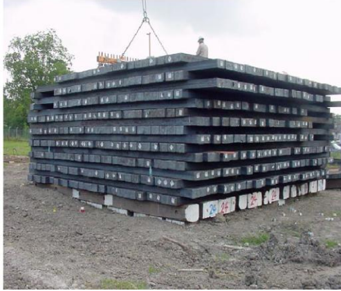
Photograph 2. One of three test cells, each with a different replacement ratio, fully loaded with 1 million kilograms of steel ( 177 \text{ kN/m}^2 ) (Cali et al., 2005).
